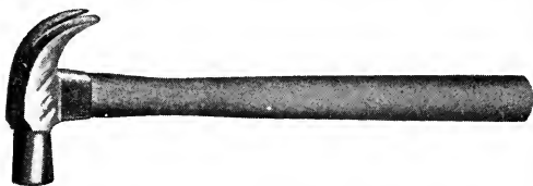
Fig. 95—Adz Eye Nail Hammer
